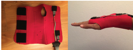
Figure 1. glove with built in inertial sensors.
