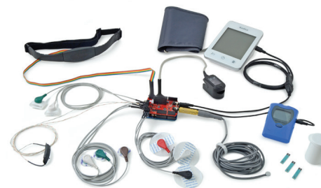
Figure 1. E-health sensor platform V2.0 for Arduino and Raspberry Pi connected to an Arduino board and all biomedical sensors.
